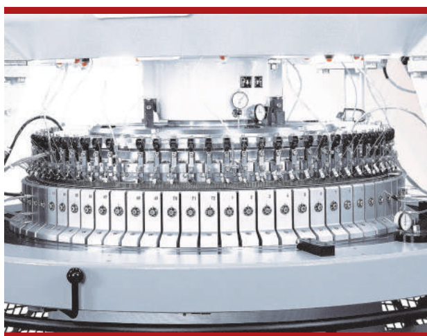
Machine head of the D4 2.2 II, a very popular interlock machine by Mayer & Cie.
