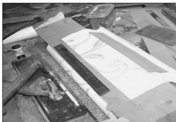
Card maker making punch cards for jacquard weaving
