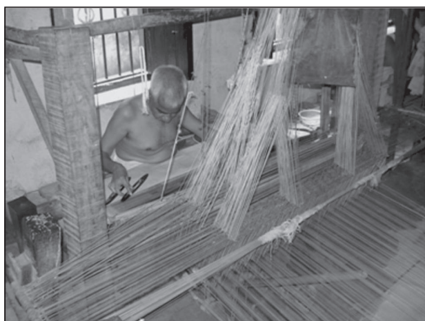
A weaver, weaving silk fabric on jacquard pit loom
