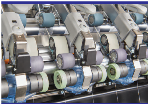
The compacting device COMPACTdrum requires five to eight watts less energy per spindle for compressing the fibers compared to compacting solutions from other suppliers.
