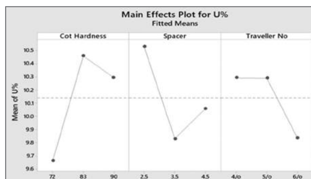
Figure 1: Effect of ring frame process variables on P/V yarn unevenness
