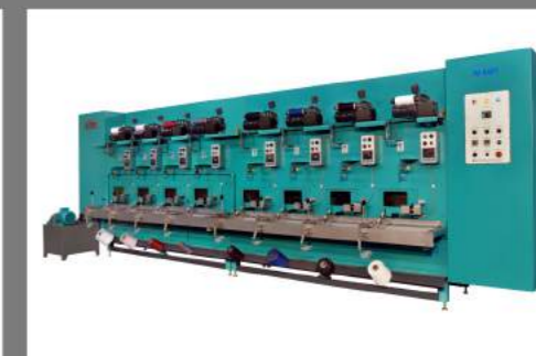
Single End Sizing RI 8001 (1-4-8 Spindles / Speed 250 MPM)
