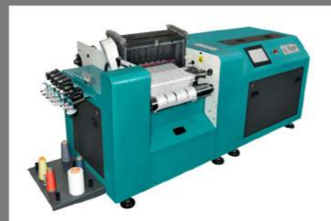
Sample Rapier Weaving Machine (50 cm / 5-30 meter / 8 colours)
