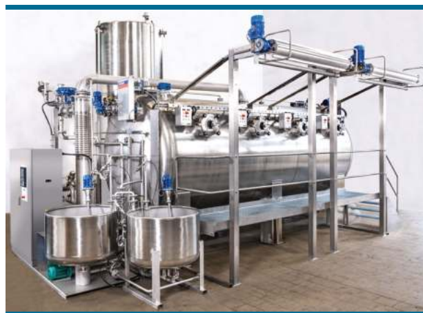
FabricMaster – fast, versatile, and economic jet dyeing machine
