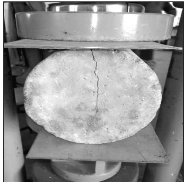
Figure 2 Experimental set up for Split Test Specimen
