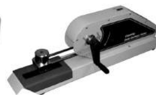
Figure 5 (5.3) : RUBBING FASTNESS TESTER
