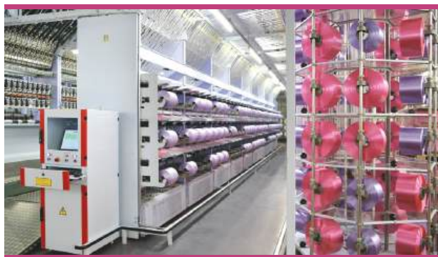
The eAFK Big V multi-spindle texturing machine is a central component of the Oerlikon Barmag product brand for manufacturing high-quality, high-titer yarns.
