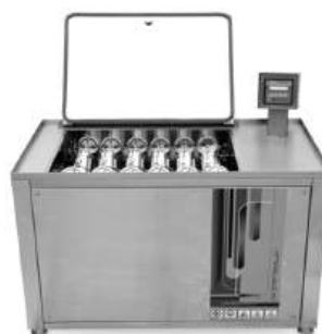
Figure 4 (5.2) : WASHING FASTNESS TESTER
