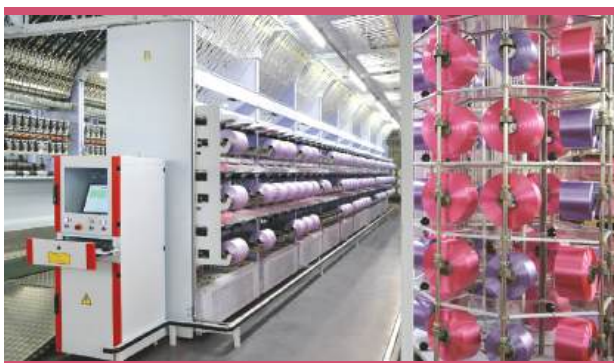
The eAFK Big V multi-spindle texturing machine is part of the solution of the Barmag product brand Oerlikon Barmag for the production of high-quality, high-titer yarns.
