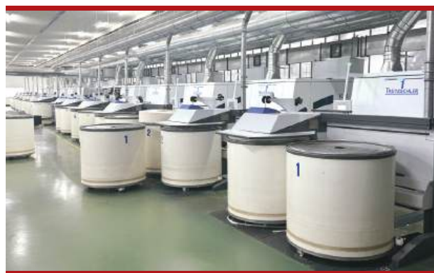
Tra Ly operates numerous Trützschler carding machines. Recently, the TC 19i completed Tra Ly's portfolio.
