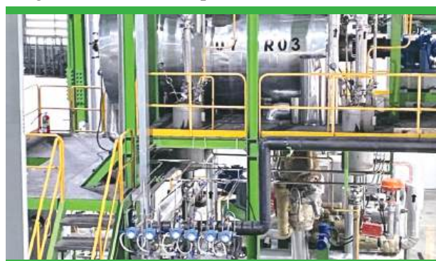
OBHE's homogenization technology stands for the thermomechanical recycling of processed post-industrial polyester waste.
