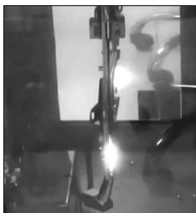
Fig. 1 - Vertical flammability test
