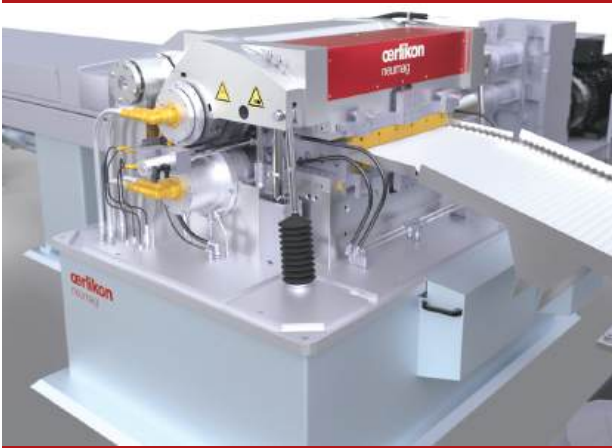
Crimping is one of the most important and demanding steps in the staple fiber process. As such, the condition of the relevant components has an impact on product quality.
