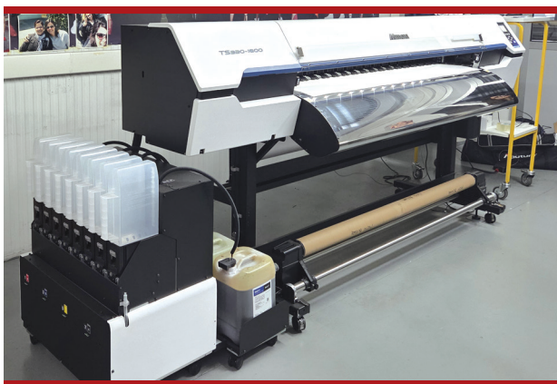
Erreà has opted for a combined Tiger600-1800TS and TS330-1600 setup to support high-volume production, colour consistency and customised sportswear manufacturing
