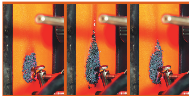
The test series demonstrates the limited flame spread. The expandable graphite swells to 40 to 60 times its original volume, forming a stable protective barrier against flames that remains effective, even after more than five minutes.
