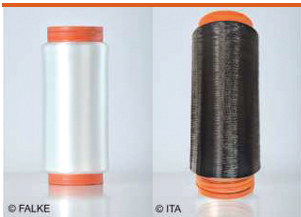
White and black 96f organic PE POY, produced by the Institute of Textile Technology at RWTH Aachen University (Source: Falke and ITA, Aachen)
