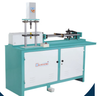
Hydraulic Cots Mounting & De-Mounting Machine
