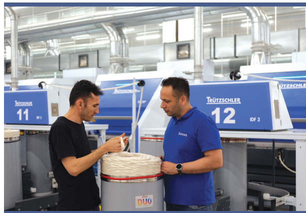
IDF 3 helps improve sliver quality, yarn evenness and strength – especially when processing higher short fiber content.
