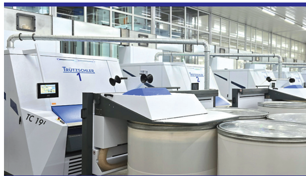
The intelligent Trützschler card TC 19i, equipped with SUPERTIP wires from Trützschler Card Clothing, ensures that every fiber is perfectly aligned, maximizing both quality and efficiency
