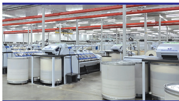
Trützschler's spinning preparation machinery transform raw cotton into a perfectly prepared sliver.
